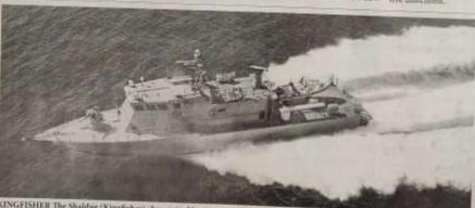
p.m. to 4 a.m. curfew KINGFISHER The Shaldag (Kingfisher) class patrol boat can reach top speeds of 30 knots and armed with missiles, automatic implemented by the guns, and cannons with a complement of 15 men. —PHOTO COURTESY OF ISRAEL SHIPYARDS
